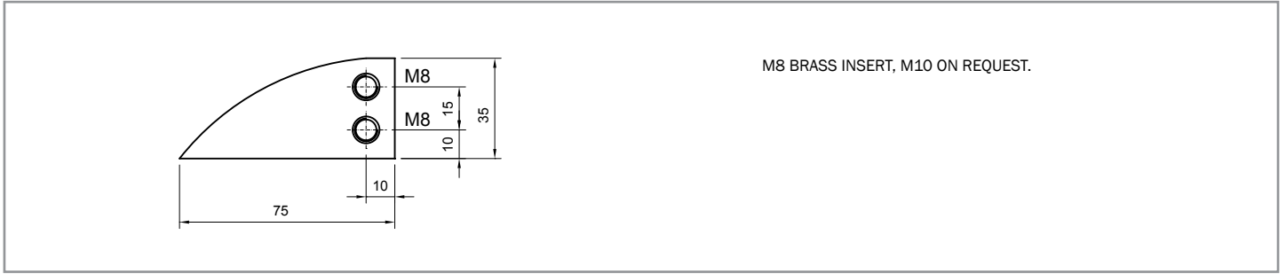
M8 brass insert, M10 on request.
